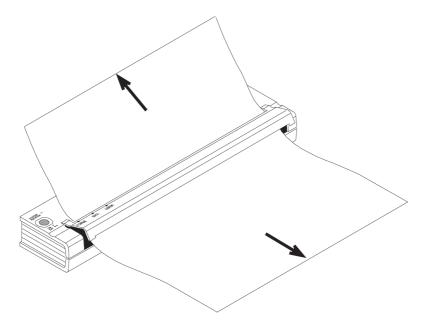
Figure 16. Pulling jammed paper out of the printer
